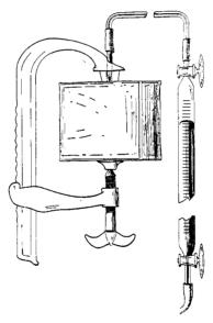
The first analyses of the gases in canned goods were effected in a Wilkinson gas analysis eudiometer. This instrument is similar in form to a Lunge's nitrometer. The graduated tube has a glass stop-cock at its upper extremity, above which is a detachable funnel. A large inverted funnel was joined to the lower end of this instrument, and the whole filled with water in a pneumatic trough. The can was punctured beneath the funnel.
